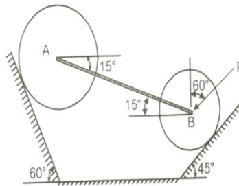
2. Determine the axial forces in the members of plane frame as shown in the below figure.
